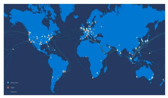
A region is a set of datacenters deployed within a latency-defined perimeter and connected through a dedicated regional low-latency network.
